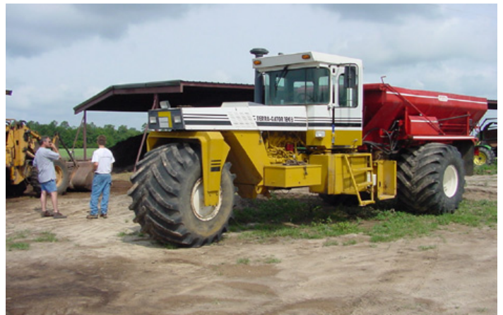
A standard agricultural manure spreader can be used to apply compost blankets on minor slopes.
